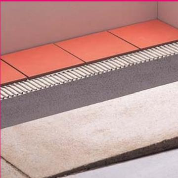
The tile bed should be sufficiently firm and free of excess adhesive prior to grouting with ARDEX-FLEX FS Flexible Tile Grout with Built-In Admix for tile joint widths up to 4mm wide or ARDEX-FLEX FL Rapid Setting Flexible Cement-Based Grouting Compound for tile joints from 3-15mm wide. If further colours are required, please consult the ARDEX C 2 data sheet\*.
