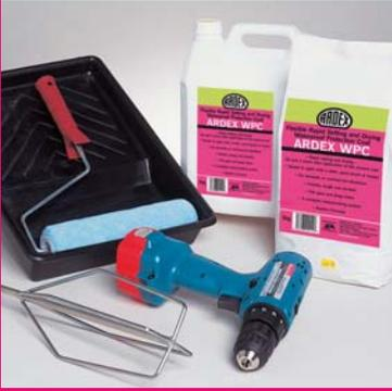
**1** Ensure that you have the appropriate tools and sufficient ARDEX WPC to cover the intended area. For coverage information refer to the technical data overleaf. The surface to be tiled must be dry, rigid, of sufficient strength and free from dust, grease, dirt, etc. Apply at temperatures above 5°C.
