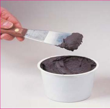
**2** **MIX NUMBER ONE** Mix a small amount of ARDEX WPC to a slump free consistency for filling holes, gaps, joints etc. For application by spatula, pallet knife or trowel, mix approximately 1.75kg ARDEX WPC liquid with 2.5kg ARDEX WPC powder per m<sup>2</sup> at 3mm thickness, i.e 4.25kg of Mix No.1 per m<sup>2</sup> at 3mm. The working time is approximately 45 minutes at 20°C.
