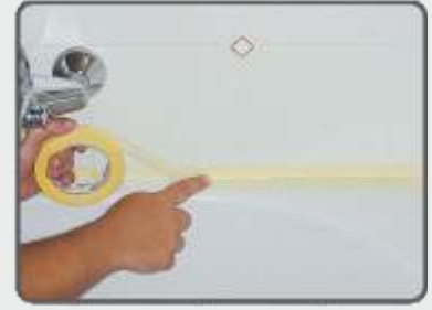
It is necessary to use adhesive tape, in order to avoid dirt during application.
